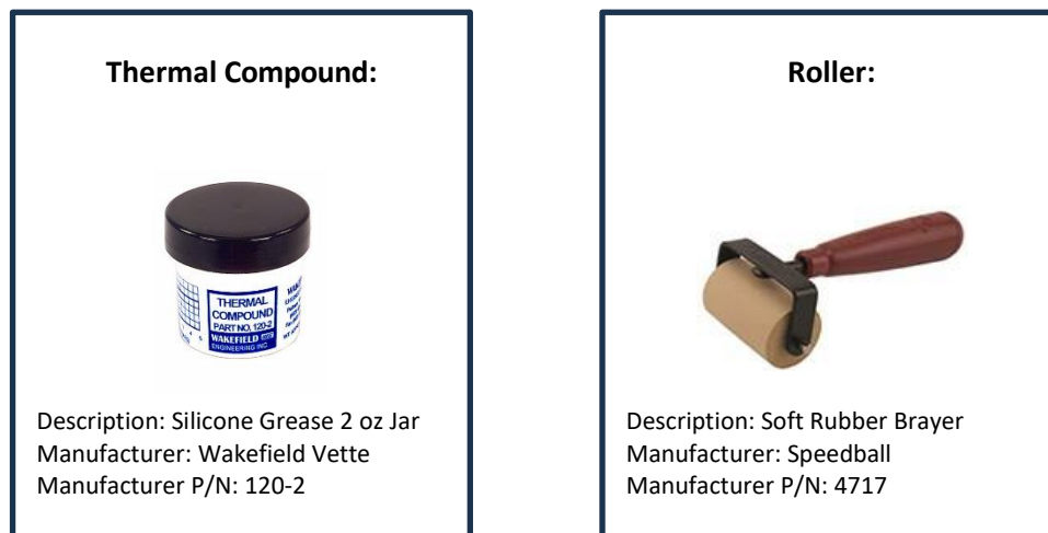
Figure 4: Recommendation for thermal compound (left) and roller (right). A roller is used to apply a thin even layer of thermal paste to the interface between the amplifier and the heat sink. Any electrically non-conductive thermal compound with at least the same thermal conductivity as the one listed should be ok to use.
