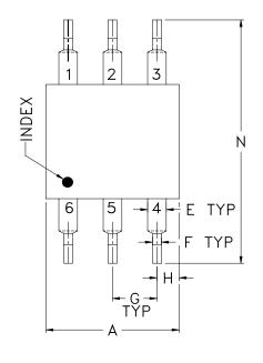
NOTE: PIN NUMBERS DO NOT APPEAR ON UNIT, FOR REFERENCE ONLY INDEX MARK INDICATES PIN 6.
