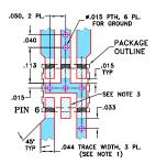
NOTES: 1. TRACE WIDTH IS SHOWN FOR ROGERS RO4350B WITH DIELECTRIC THICKNESS .020" ± .0015"; COPPER: 1/2 0Z. ON EACH SIDE. FOR OTHER MATERIALS TRACE WIDTH MAY NEED TO BE MODIFIED. 2. BOTTOM SIDE OF THE PCB IS CONTINUOUS GROUND PLANE.
