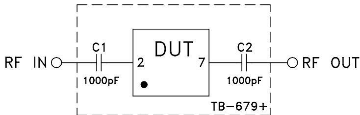
**Fig. 1.** Block Diagram of Test Circuit used for characterization. Mini-Circuits test board TB-679+. Insertion loss, return loss, and VSWR measured using Agilent N5230A network analyzer. Performance at frequencies below 30 MHz may be improved by increasing capacitance at C1 and C2. Depending on application requirements, this device may be effective at frequencies up to 10 GHz.
