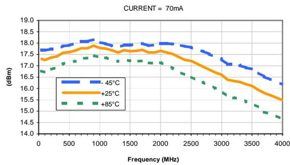
**OUTPUT POWER at 1dB Compression vs. CURRENT**
