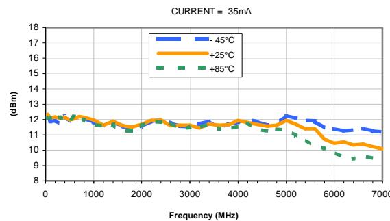
OUTPUT POWER at 1dB Compression vs. CURRENT
