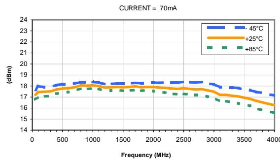
OUTPUT POWER at 1dB Compression vs. CURRENT
