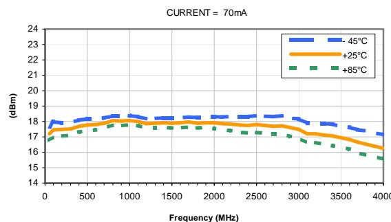
OUTPUT POWER at 1dB Compression vs. CURRENT
