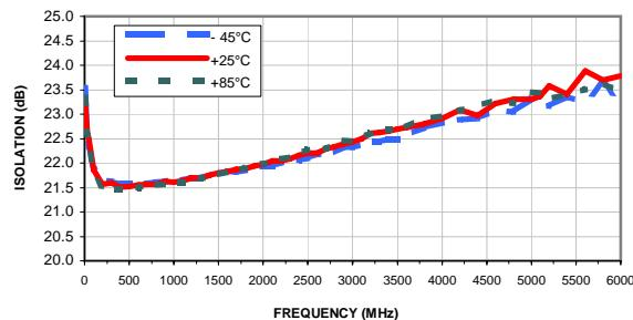
**ISOLATION vs. FREQUENCY & DEVICE VOLTAGE**
