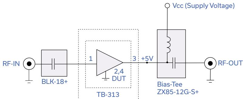
Fig 1. Block Diagram of Test Circuit used for characterization. (DUT soldered on Mini-Circuits Characterization test board TB-313) Gain, Return loss, Output power at 1dB compression ( $P_{1\text{ dB}}$ ) , output IP3 (OIP3) and noise figure measured using Agilent's N5242A PNA-X microwave network analyzer.
