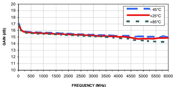
**GAIN vs. FREQUENCY & DEVICE VOLTAGE**
