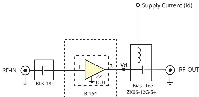
**Fig 1.** Block Diagram of Test Circuit used for characterization. (DUT soldered on Mini-Circuits Characterization test board TB-154)
