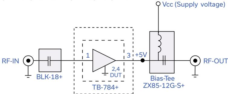
Fig 1. Block Diagram of Test Circuit used for characterization. (DUT soldered on Mini-Circuits Characterization test board TB-784+) Gain, Return loss, Output power at 1dB compression (P1 dB), output IP3 (OIP3) and noise figure measured using Agilent's N5242A PNA-X microwave network analyzer.
