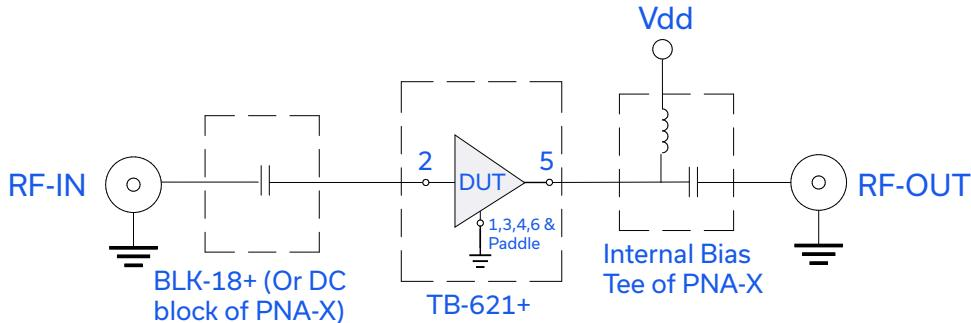
Fig 1. Characterization Circuit
