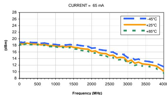
OUTPUT POWER at 1dB Compression vs. CURRENT
