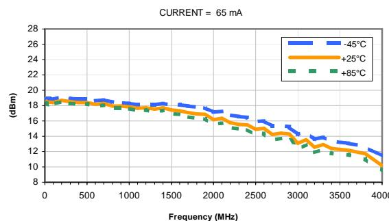
OUTPUT POWER at 1dB Compression vs. CURRENT
