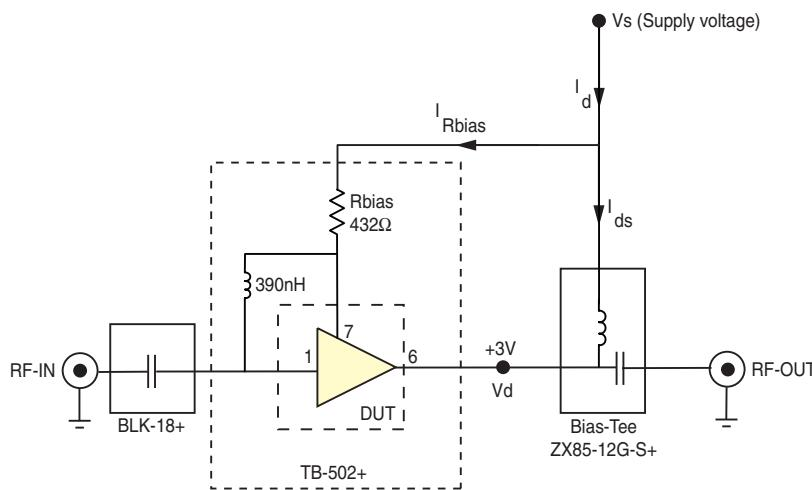
**Fig 1.** Block Diagram of Test Circuit used for characterization. (DUT soldered on Mini-Circuits Characterization Test Board TB-502+) Gain, Output power at 1dB compression (P<sub>1dB</sub>), Output IP<sub>3</sub> (OIP<sub>3</sub>) are measured using R&S Network Analyzer ZVA-24. Noise Figure measured using Agilent's N5242A PNA-X microwave network analyzer.
