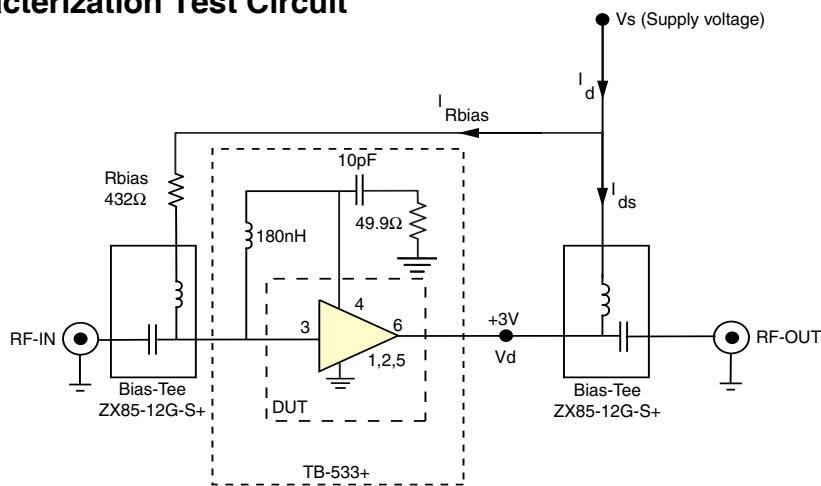
**Fig 1.** Block Diagram of Test Circuit used for characterization. (DUT soldered on Mini-Circuits Characterization Test Board TB-533+) Gain, Return loss, Output power at 1dB compression ( $P_1$  dB), Output IP3 (OIP3) and Noise Figure measured using Agilent's N5242A PNA-X microwave network analyzer.
