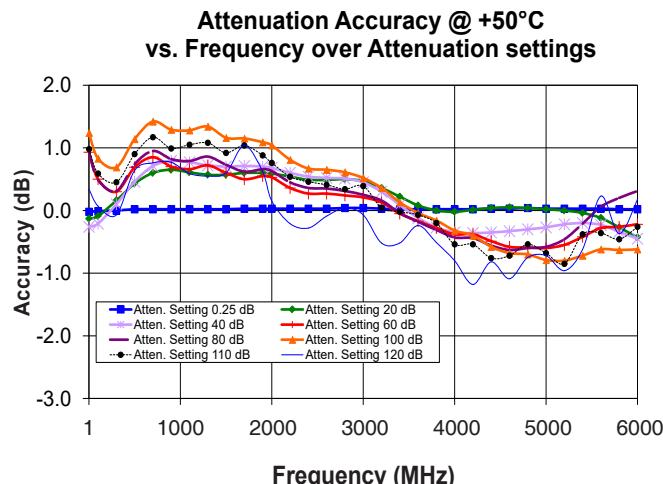
**Attenuation relative to Insertion Loss @ +50°C vs. Frequency over Attenuation settings**
