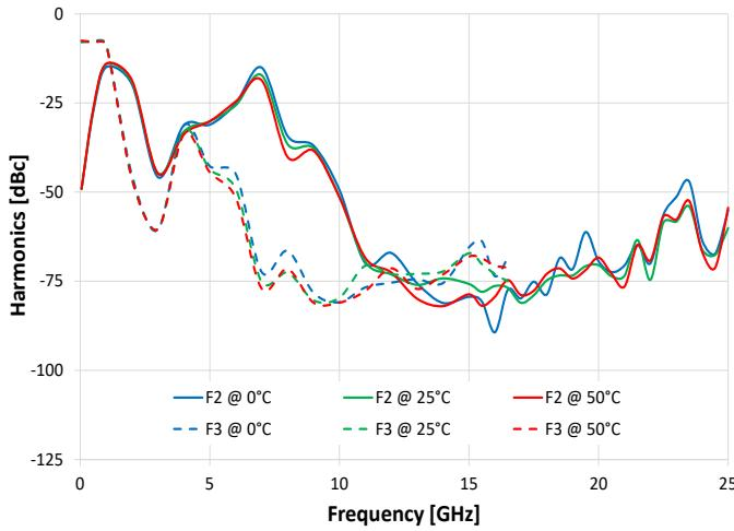
Sub-Harmonics vs. Output Frequency @ -20 dBm
