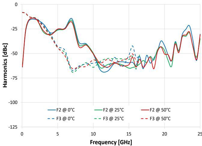
Sub-Harmonics vs. Output Frequency @ -45 dBm
