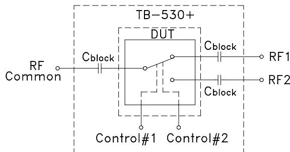
Figure 1: Block Diagram Of Test Circuit Used For Characterization.
