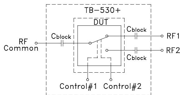
Fig. 2: Evaluation board includes case, connectors and components soldered to PCB.
