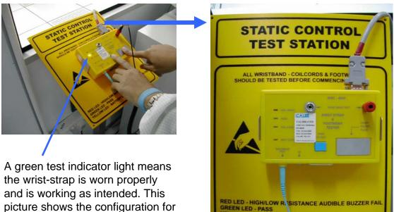
picture shows the configuration for testing wrist-straps. The test station can also be configured to test antistatic footwear.
