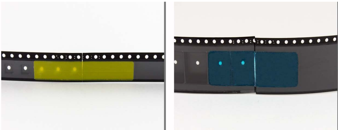
Figure 1: flat leader/trailer tape spliced onto carrier tape with pockets.
