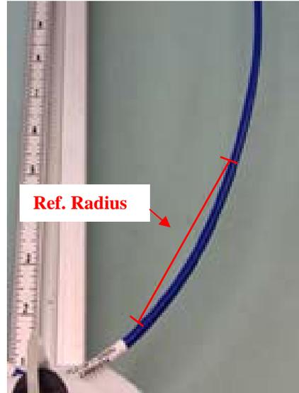
*Figure 2: 3ft. Flexible Test Cable attached to the Cable Flexure Test Fixture at its reference start position*
