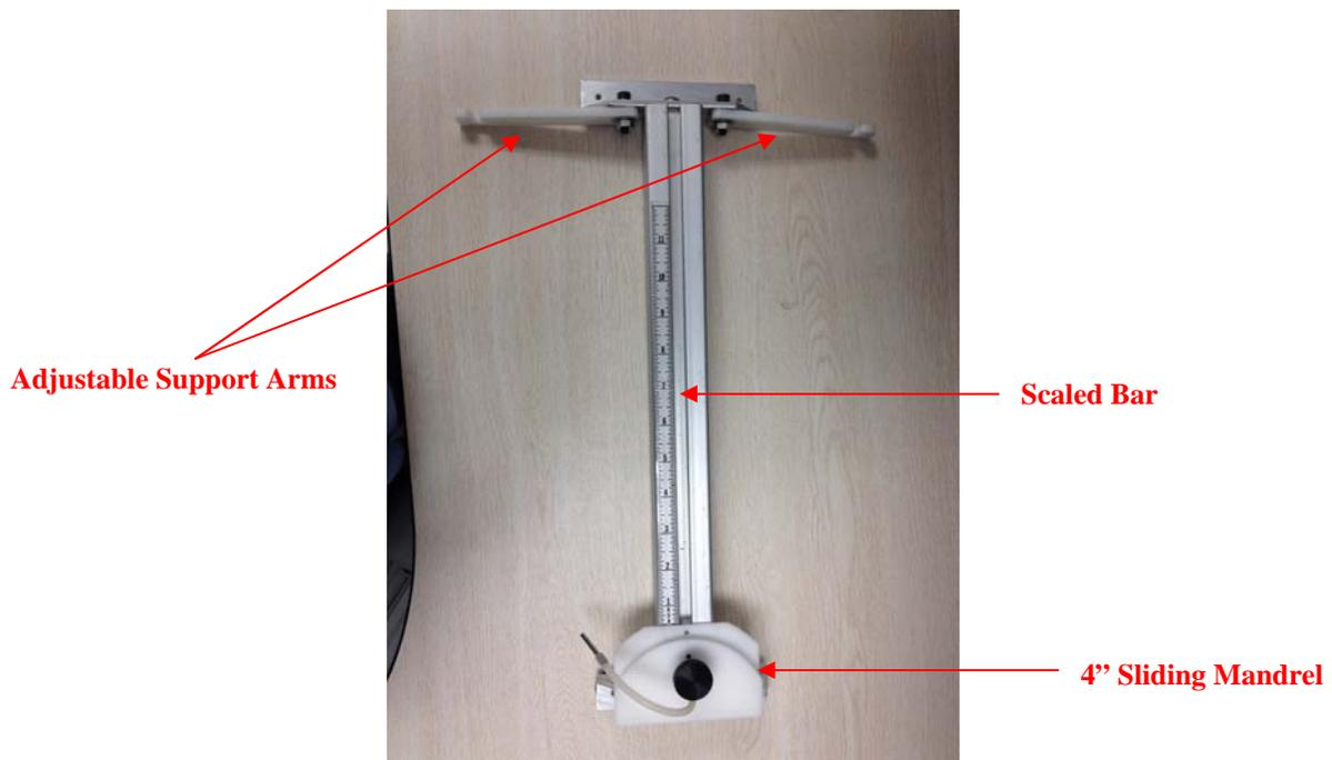
Figure 1: Cable Flexure Test Cable (MCL P/N: B85-L26000-00)
