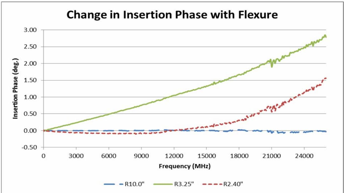
*Figure 8: Change in Insertion Phase with flexure in reference to start position*
