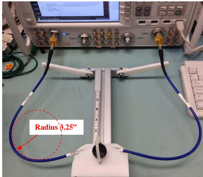
*Figure 4: 3ft. Flexible Test Cable with a bend radius of 3.25"*
