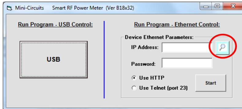
After clicking on the search icon, the IP search will pop up with a list of smart power meter IP addresses found and their HTTP ports on the left side of the screen, and full details of each unit on the right. Mark the IP address you wish to use and click select. The search window will close, and the IP address and port will be entered in the IP address field of the initial screen automatically.
