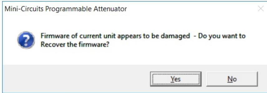
*Firmware – recovery option (except PWR-40PW-RC or PWR-8PW-RC)*
