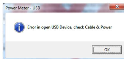
After acknowledging the alert, the main measurement screen will appear with no unit selected and a 'Not Connected' notice. Click on 'reset connection' to try connecting again, or close the program.
