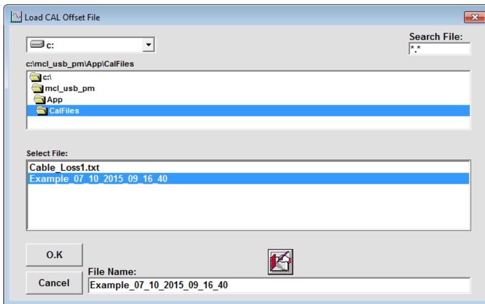
To create an offset file manually click on the edit icon over the file name window and a sample offset file will be created. Replace the values in the sample file with the values you need and save the file. There is no requirement for any specific file name or suffix, however as the file is a simple text file saving it with a txt suffix to simplify future editing is recommended.
