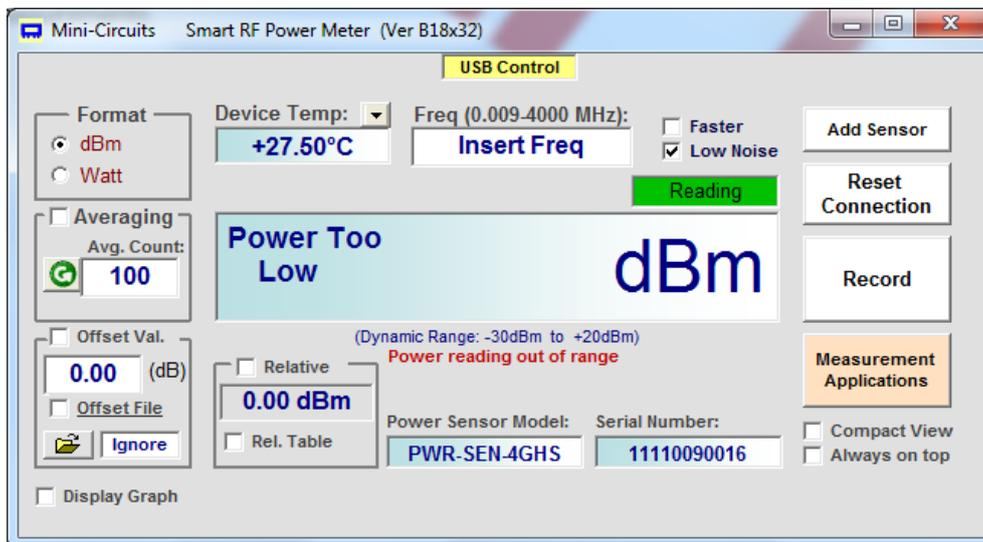
If multiple PWR power sensors are connected to the computer via USB, the initial screen will show a list of S/N for connected units. You can select a single unit, or multiple units you wish to start with – each opening in its own window. The program can handle up to 24 units connected simultaneously.
