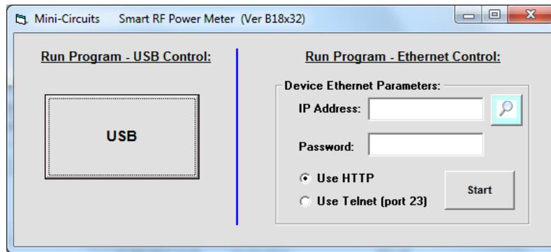
The startup window allows you to select the control method you wish to use for the PWR units, USB or Ethernet control. All models support USB control, only models with an 'RC' suffix such as PWR-8GHS-RC support Ethernet control. For USB control click on the USB button, for Ethernet control see section 5.2.
