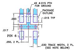
NOTES: 1. TRACE WIDTH IS SHOWN FOR ROGERS RO4350B WITH DIELECTRIC THICKNESS 0.030"  $\pm$  0.002"; COPPER: 1/2 OZ. EACH SIDE. FOR OTHER MATERIALS TRACE WIDTH MAY NEED TO BE MODIFIED.
