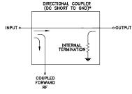
ELECTRICAL SCHEMATIC IS FOR DIRECTIONAL COUPLER WITH INTERNAL TRANSFORMER(S) THA ROUTES DC FROM RF PORTS TO GROUND.
