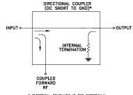
ELECTRICAL SCHEMATIC IS FOR DIRECTIONAL COUPLER WITH INTERNAL TRANSFORMER(S) THA POLITES DC FROM RF PORTS TO GROUND
