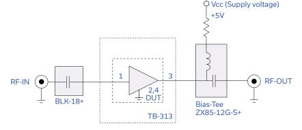
Fig 1. Block Diagram of Test Circuit used for characterization. (DUT soldered on Mini-Circuits Test Board TB-313)
