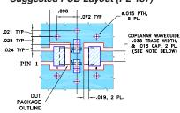
COPLANAR WAYEGUIDE PARAMETERS ARE SHOWN FOR ROGERS ROA\$50B WITH THICKNESS .020" ± .0015". COPPER: 1/2 02. EACH SIDE. FOR OTHER MATERIALS TRACE WIDTH & GAP MAY NEED TO BE MODIFIED. NOTES: 1.
