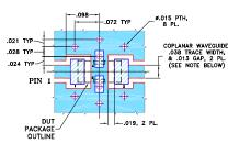
NOTES: 1. COPLANAR WAVEGUIDE PARAMETERS ARE SHOWN FOR ROGERS ROASSOB WITH THICKNESS 0.20" ± .0.015". COPPER: 1/2 0.2 EACH SIDE. FOR OTHER MATERIALS TRACE WIDTH & GAP MAY NEED TO BE MODIFIED.
