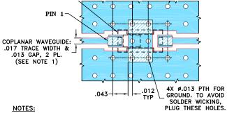
1. TRACE WIDTH AND GAP ARE SHOWN FOR ROGERS RO4350B WITH DIELECTRIC THICKNESS .010" ± .001". COPPER: 1/2 OZ. EACH SIDE. FOR OTHER MATERIALS TRACE WIDTH AND GAP MAY NEED TO BE MODIFIED.
