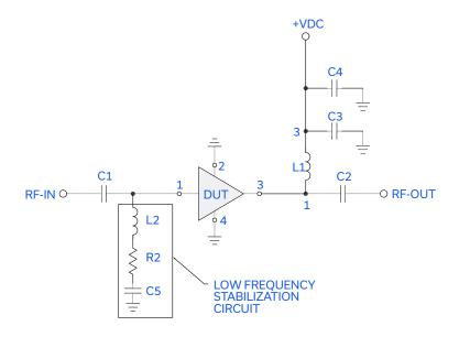
Fig 2b. Evaluation board TB-761-103+ unconditionally stable (see note AN-60-064)
