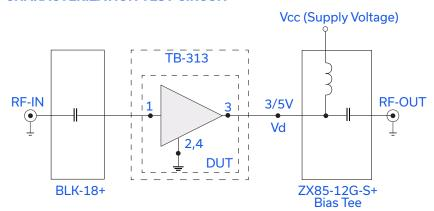
Fig 1. Block Diagram of Test Circuit used for characterization. (DUT tested on Mini-Circuits Characterization test board TB-313)
