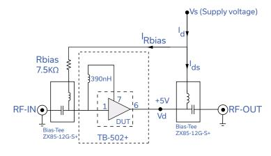
Fig 1. Block Diagram of Test Circuit used for characterization. (DUT soldered on Mini-Circuits Characterization Test Board TB-502+) Gain, Output power at 1dB compression (P1dB), Output IP3 (OIP3) and Noise Figure measured using Agilent's N5242A PNA-X Microwave network analyzer.
