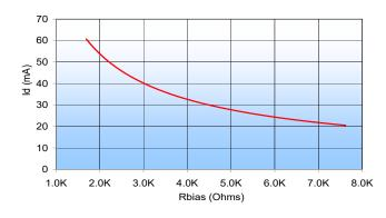
Fig 4. Id varies as a function of Rbias. The Id current range is defined based upon the specific Rbias value noted in the Application Circuit (Fig 3). Rbias may be adjusted to optimize Id for a customers' application. RF performance will vary accordingly.
