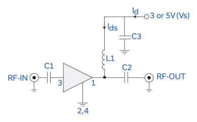
Fig 2. Recommended Application Circuit Note: Resistance of L1, 0.1- $0.2\Omega$  typically
