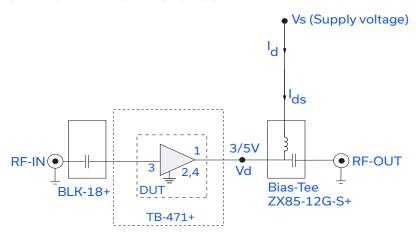
Fig 1. Block Diagram of Test Circuit used for characterization. (DUT soldered on Mini-Circuits Characterization Test Board TB-471+)
