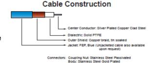
er Pin: Sliver Plated Copper Clad Stee
