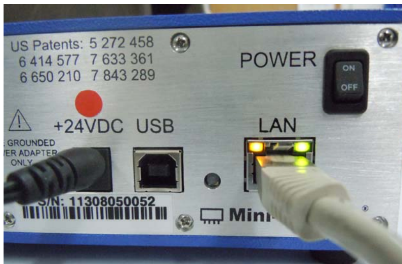
Figure 2.3.3b: switch matrix power & Ethernet control connections
