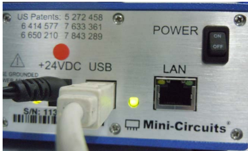
Figure 2.3.2b: switch matrix power & USB control connections
