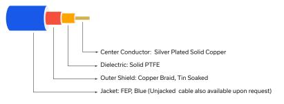
Connectors: Coupling Nut: Stainless Steel, Passivated Body: Brass, Gold Plated Center Pin: Beryllium Copper, Gold Plated
