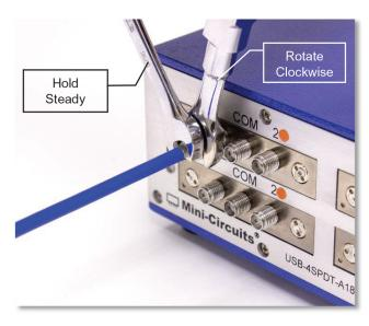
\*NOTE: Mini-Circuits recommends using a 5/16-inch open end wrench calibrated to 8 inch-pounds maximum torque to prevent damage due to over-torqueing the connector.
