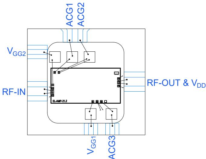
Figure 5. AVA-223MP-D+ Assembly Diagram
