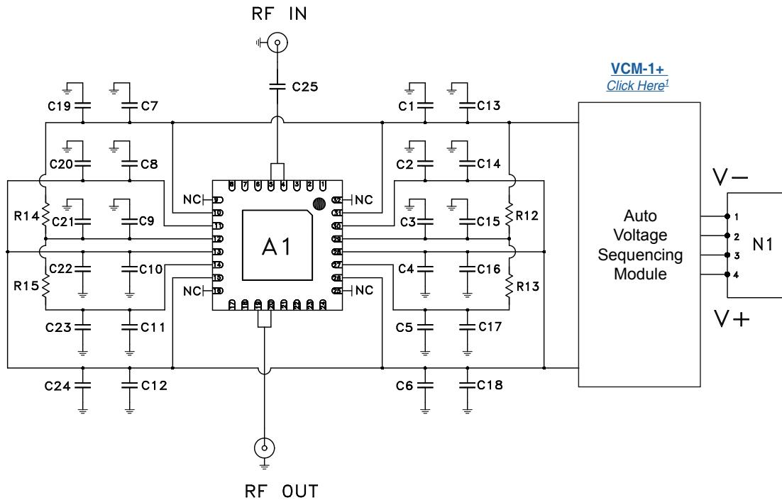
**Fig. 1 Schematic of Test Board TBD (Test & Application)**
