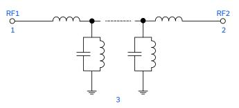
Figure 1. BFHKI-9901+ Functional Diagram
