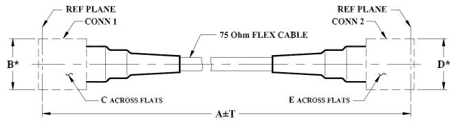
\* OVERALL CONNECTOR OR CABLE & BOOT DIMENSION (CONNECTOR SHAPE MAY VARY)
