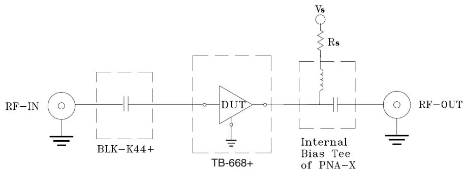
Fig 1. Characterization Circuit
