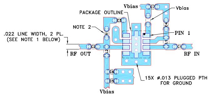
NOTES: 1. TRACE WIDTH IS SHOWN FOR ROGERS RO4350B WITH DIELECTRIC THICKNESS  $.010" \pm .001"$ ; COPPER: 1/2 OZ. EACH SIDE. FOR OTHER MATERIALS TRACE WIDTH MAY NEED TO BE MODIFIED.
