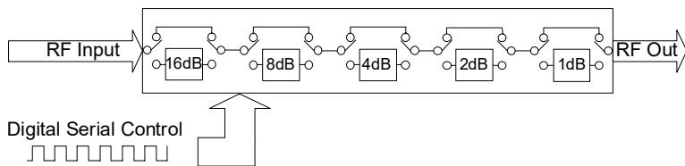
The DAT-31A-SN+ serial interface consists of 5 control bits that select the desired attenuation state, as shown in Table 1: Truth Table
