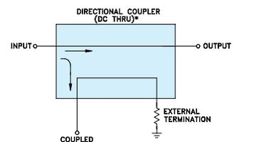
\* ELECTRICAL SCHEMATIC FOR DIRECTIONAL COUPLERS REQUIRING EXTERNAL TERMINATION THAT IS DESIGNED WITHOUT INTERNAL TRANSFORMERS.
