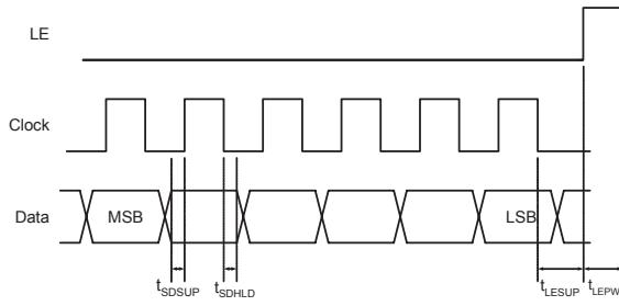
**Figure 2. Serial Interface Timing Diagram****Table 3. Serial Interface AC Characteristics**
