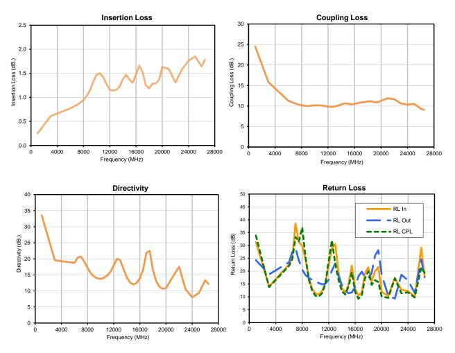
Note: Testdata of Die packaged in 4x4 mm, 24-lead MCLP package
