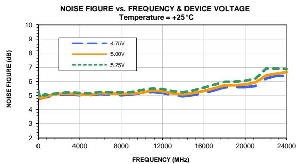
Note: Test data of Die packaged in 4-lead ceramic package
