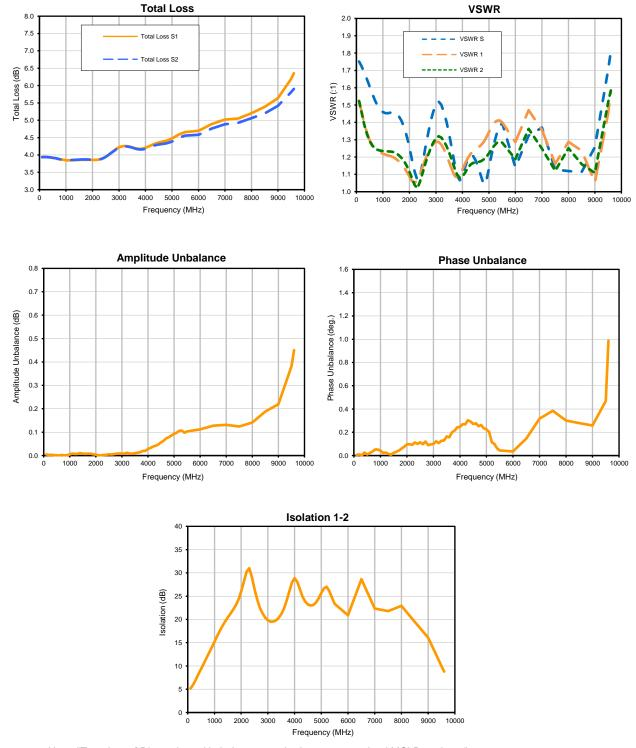
Note: "Test data of Die packaged in industry standard, 5x5 mm, 32-lead MCLP package"
