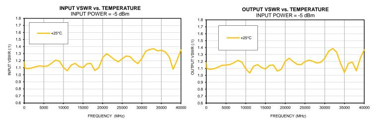
Note: Test data of Die packaged in industry standard 2x2mm 6-Lead MCLP Package
