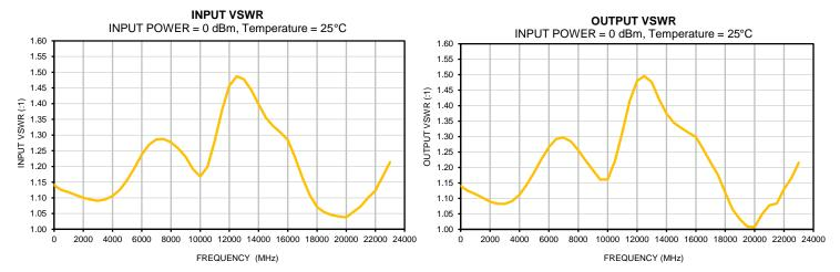
Note: Test data of Die packaged in industry standard 2x2mm 8-Lead MCLP Package
