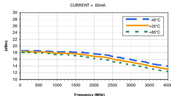
OUTPUT POWER at 1dB Compression vs. CURRENT
